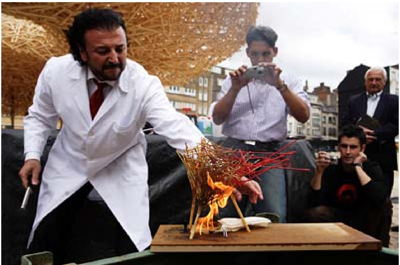
After being protected, the prototype was impregnated with gasoline and fired, but it could not be burned
