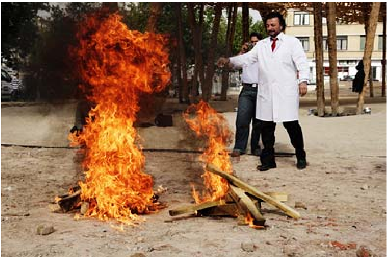
Samples of the wood used to build the structure of the Cityscape were taken to demonstrate the effectiveness of the AyDo AquaElix Flame Safe. The pile at the right was protected and as you see it doesn't burn. The pile to the left was not protected and the wood was completely burned. Notice the difference in the flame of both piles.
