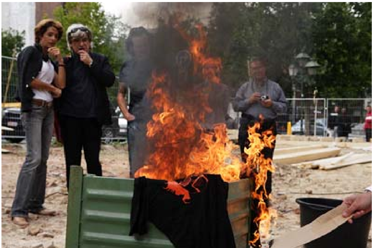
AyDo AquaElix Flame Safe showing another aspect of its performance. On the back one t-shirt was first protected with the Flame Safe, after wet with abundant gasoline and finally fired. The piece remained intact after the gasoline was completely burned. The t-shirt in front on the picture was first wet with regular water, after with gasoline and finally fired. The piece was completely reduced to ashes.
